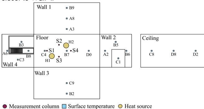
Figure 8 Sensor location in test room.
