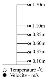
Figure 9 Measurement column heights of thermocouples and velocity sensors.
