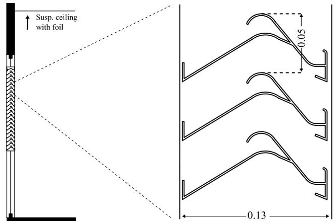
Figure 7 Louvre installation in test room wall (left) and close up of three regular louvre elements (right).
