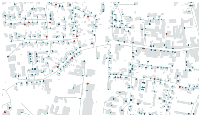
Figure I.2: Example of metering on a distribution network. Each coloured point is a flow meter displaying the network data where red points show there is an issue in the network. Figure adapted from [9].
