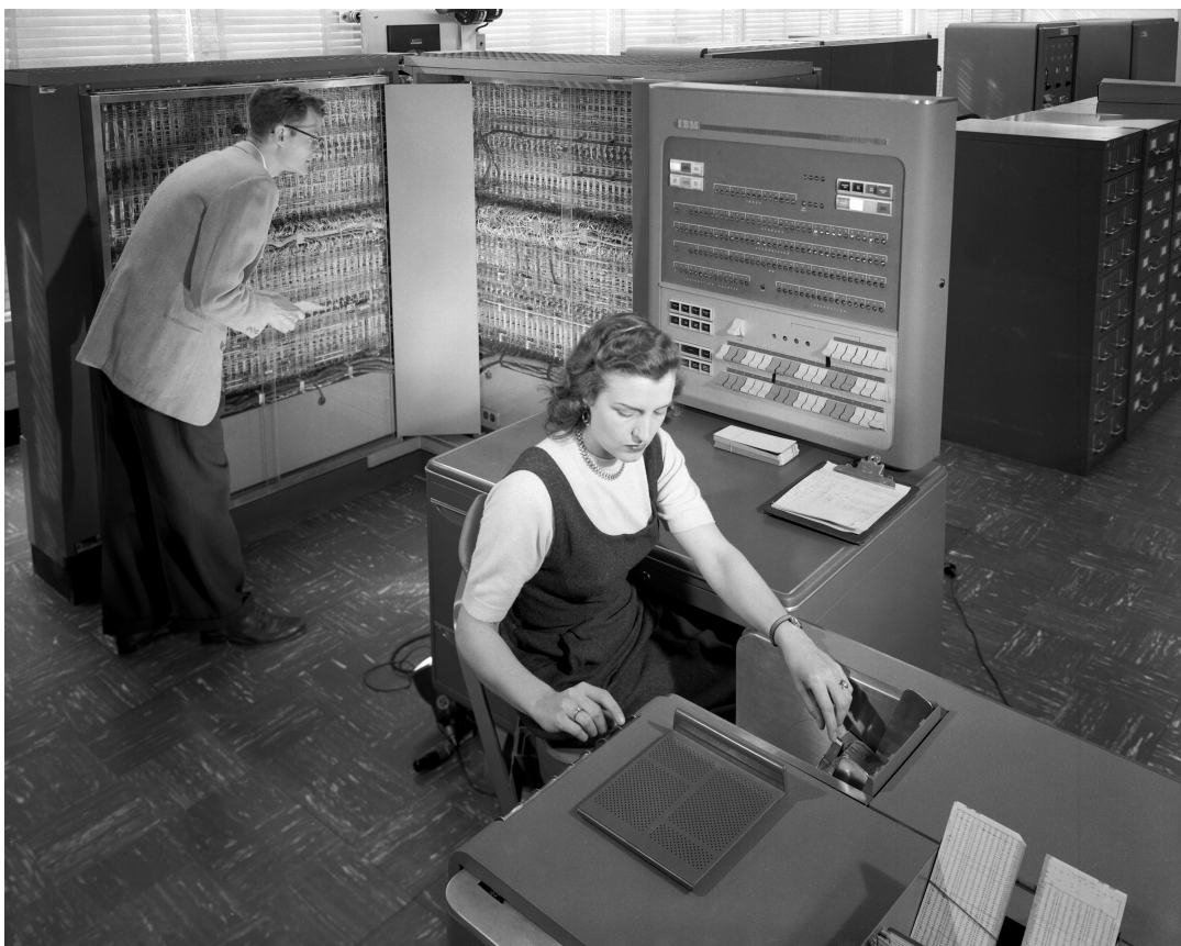
FIGURE 5.3: Woman operating an IBM 711 card reader on an IBM 704 computer in 1957. IMAGE SOURCE: “IBM 704 computer at NACA” by NASA. Retrieved from https://commons.wikimedia.org/wiki/File:IBM_Electronic_Data_Processing_Machine_-_GPN-2000-001881.jpg . License: Creative Commons Public Domain
