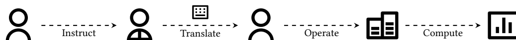
FIGURE 5.4: The programmer writes the program which is then translated by the coder into physical cards. These cards are fed to the card reader by the machine operator at which point computations are performed.
