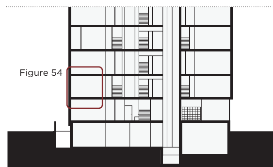
Figure 53 Basic information about the project (left) and principle section from before the renovation (right) (based on Lacaton & Vassal n.d.). The red square indicates the focus of Figure 54.
