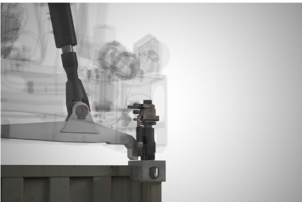
Stinis shock absorbing system ( https://www.stinis.com/unique-features/ )
