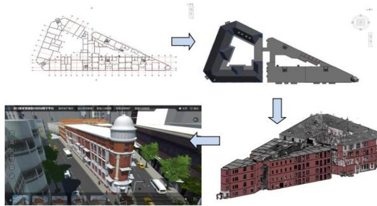
Figure 4: BIM modeling process of "Bagong House".
