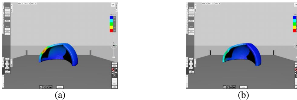
Figure 8: (a) Deformed configuration with highlighted displacements as well as (b) Deformed configuration with visualised von Mises stresses.
