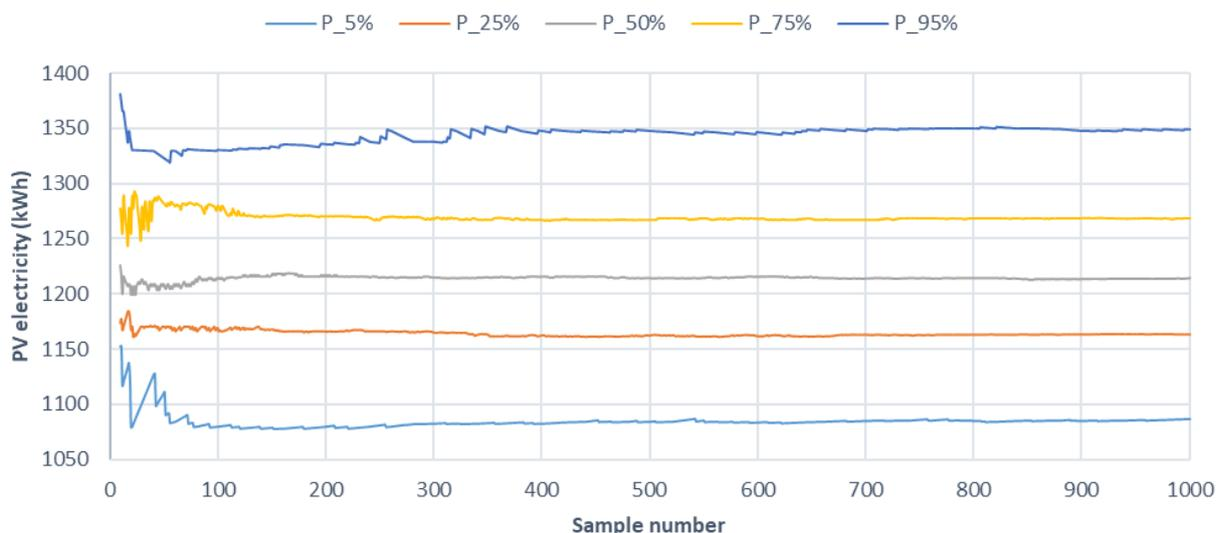
Figure 3: Stability of percentiles of electricity generated by PV systems with the sample number for the ventilation mode using the TRNSYS model.
