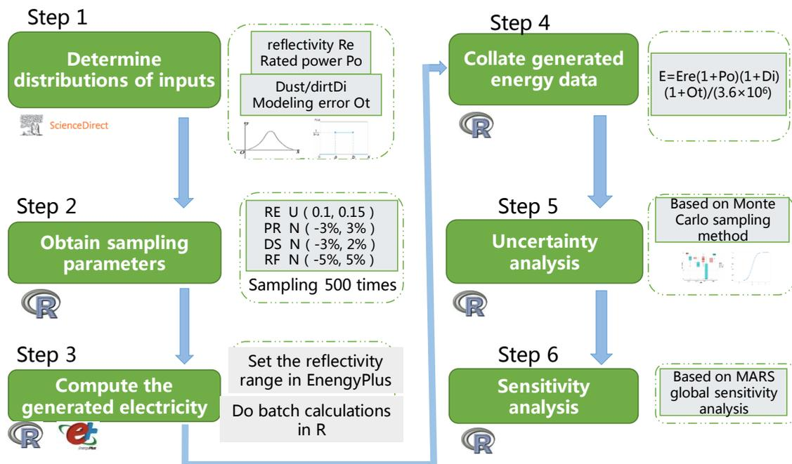
Figure 1: Flow chart of uncertainty and sensitivity analysis of building-integrated photovoltaics.
