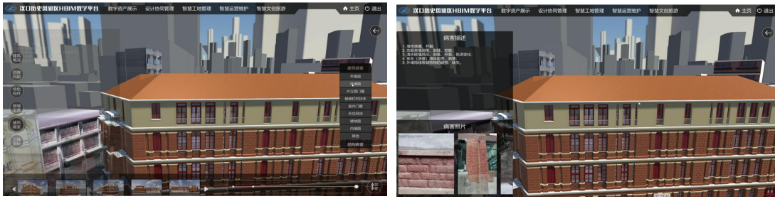
Figure 7: Snapshot of pathology database of "Bagong House" (Classify the pathologies existing in "Bagong house" according to the classification standards, and store the pathology data in the database. Click the pathology name in the list on the right to view the corresponding photos, coordinates, disease description, etc ).
