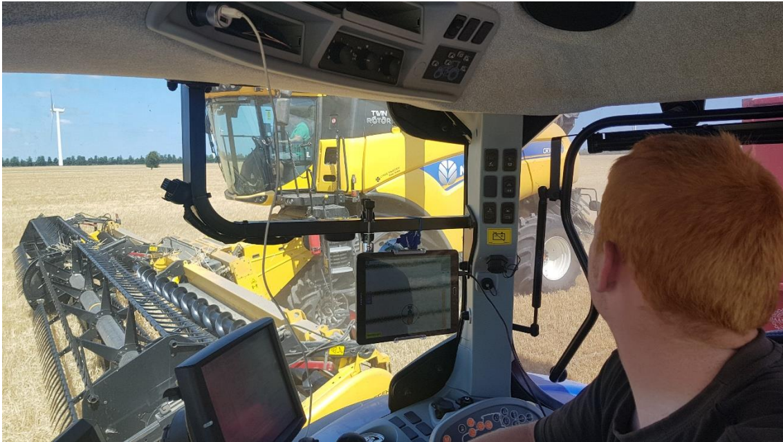
Figure 14. Android tablet in the cabin indicating and monitoring a load transfer into a grain cart.
