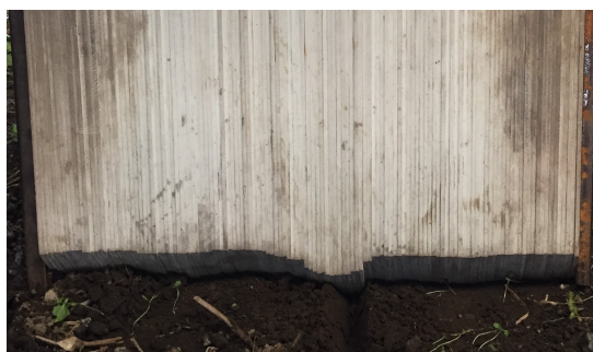
Figure 4. The analogue measurement using pinboard of the furrow in loamy sand at 40 mm irrigation.
