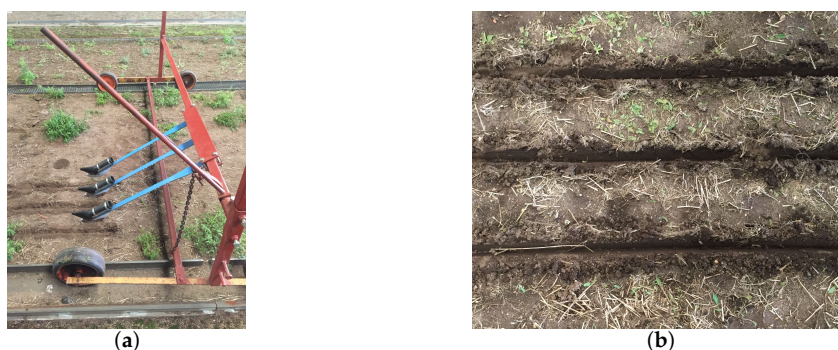
Figure 2. Frame with three of the Bomech trailing shoes (a) and three furrows in coarse sand at 40 mm irrigation (b).
