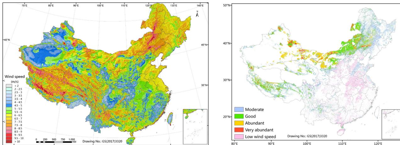
**Figure 2** Spatial distribution of (a) annual mean wind speeds and (b) exploitable wind energy resources at 100 m above ground across China.
