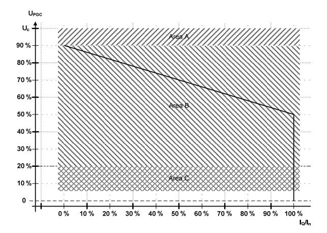
Figure 3 Requirement for reactive power supply during voltage drops (for wind turbine with an installed capacity > 1.5 MW) (Energinet 2016).
