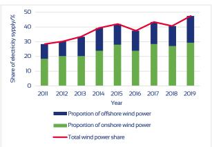
Figure 2 Proportion of onshore and offshore wind power and the total wind-power share of electricity supply in Denmark (Source: Energy Watch 2019)
