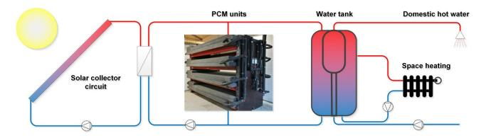
Figure 3 Demonstration of a solar combi system with heat-storage units utilizing stable supercooling of SAT (Englmair et al. 2019)
