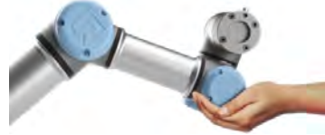
FIGURE 1.2: Lead-through programming of a Universal Robots UR3e manipulator.
