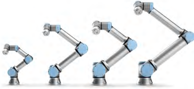
FIGURE 1.4: Universal Robots' e-Series robots, from left to right; UR3e, UR5e, UR16e, and UR10e, named after their rated payload in kilograms. 4
