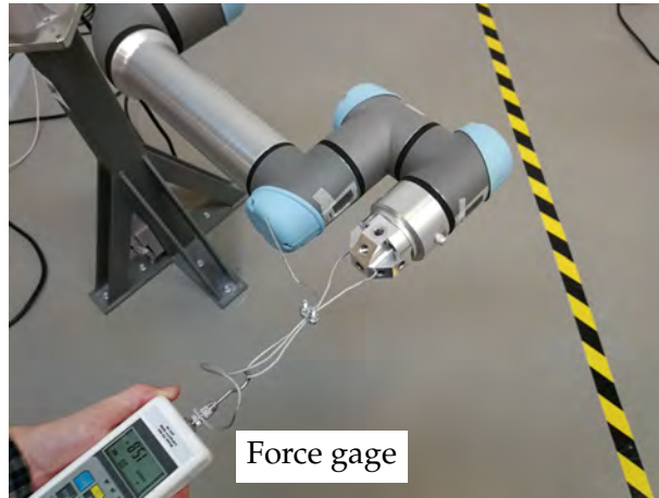
FIGURE 3.1: Experimental setup for offline identification of the joint stiffness of the Universal Robots UR5e robot.
