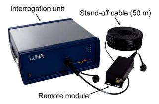
Figure 1 ODiSI-B measurement system (Luna 2017)
