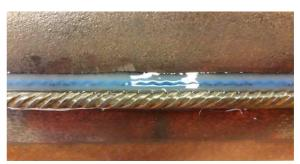
Figure 2. Installation of strain DFOS on the steel piles.
