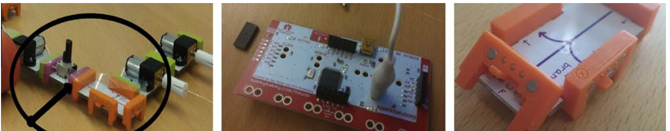
Figure 11. Left: Tape being used to hold the magnetic connectors together. Center: Broken bit connector. Right: Broken bit connector.
