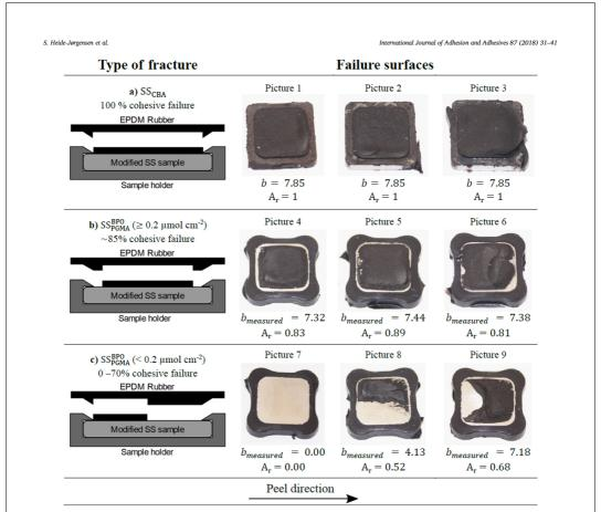
Fig. 9. Failure surfaces of various samples after peeling. a)  $SS_{CBA}$  samples with 100% cohesive fracture. b)  $SS_{PGMA}^{BPO}$  samples with the characteristic non-bonded strip along the edges. c)  $SS_{PGMA}^{PPO}$  samples with varying  $A_r$ .
