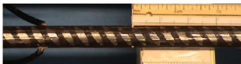
Figure 2.15: An almost smooth bar where ribs are grounded of, reprint from [16]
