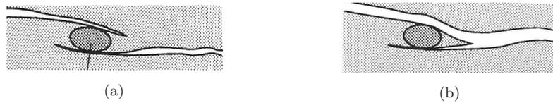
Figure 2.3: Crack-face bridging: (a) Overlapping cracks with load transfer through the aggregate, (b) Failure due to joining of cracks, reprint from [3]
