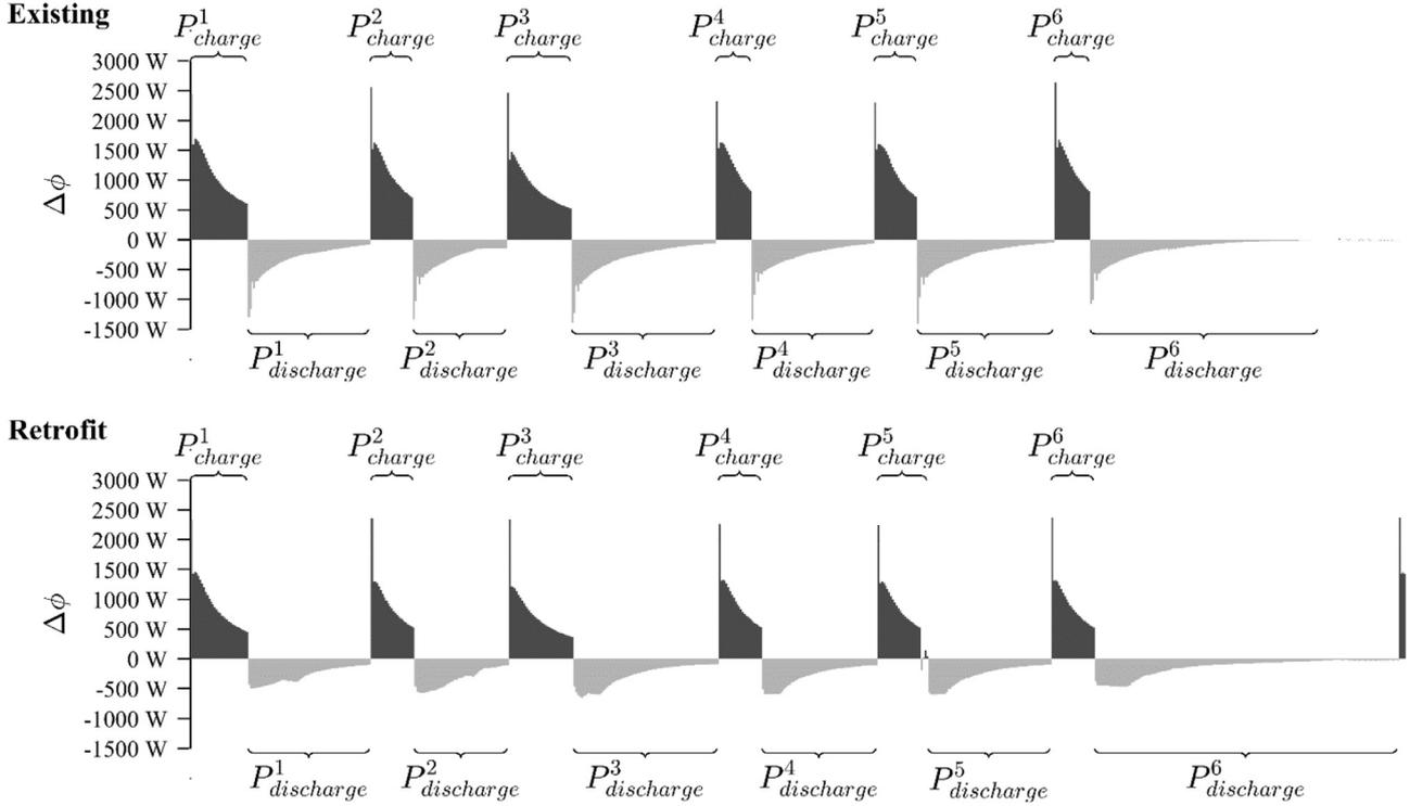
Fig. 12. Absolute shifting potential for the existing and retrofitted building using MPC setup (b).
