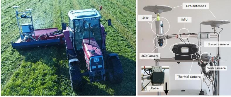
Figure 2.1: Recording platform. Reprinted from Kragh et al. (2017).
