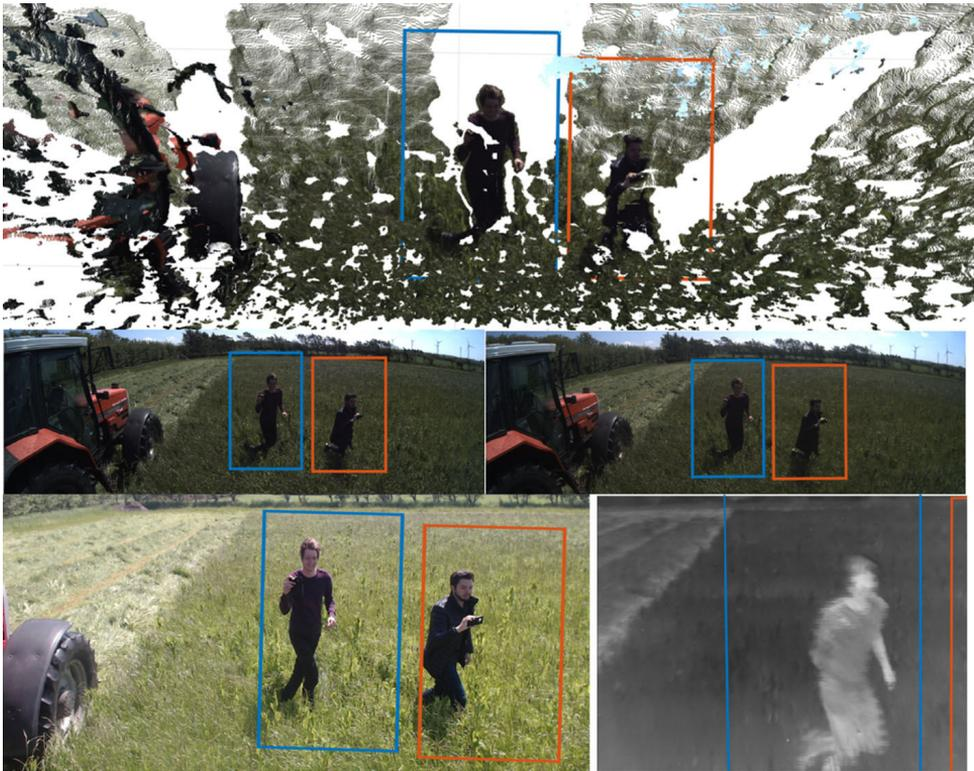
**Fig. 8** Annotations in the *left image* are projected onto the stereo point cloud (*top*). These annotations are then projected to the right and left stereo camera (*middle left and right*), the webcam (*bottom left*) and the thermal camera (*bottom right*)
