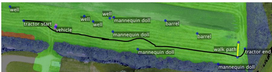
Figure 5. Orthophoto with static objects, tractor trajectory (black line) and human walk path (yellow line). An overlay shows the ground truth of vegetation (blue), ground (green) and non-traversable ground (red).
