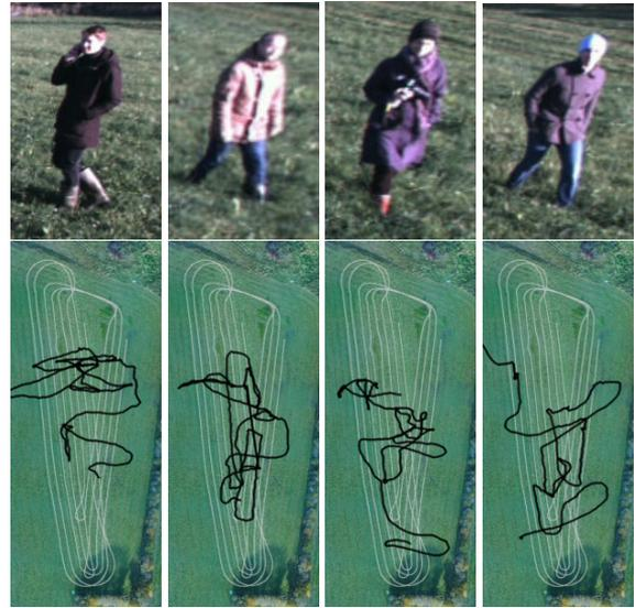
(8b) Examples of moving obstacles (from the stereo camera) and their paths (black) overlaid on tractor path (grey).
