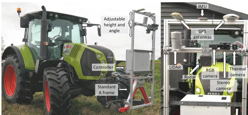
Fig. 1. Sensor platform mounted on tractor.
