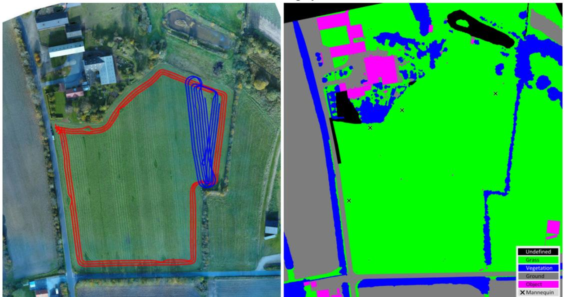
(8c) Colored and labeled orthophotos. Left: orthophoto with tractor tracks overlaid. The red track includes only static obstacles, whereas the blue track also has moving obstacles. Right: annotated orthophoto with pixel-wise labels.
