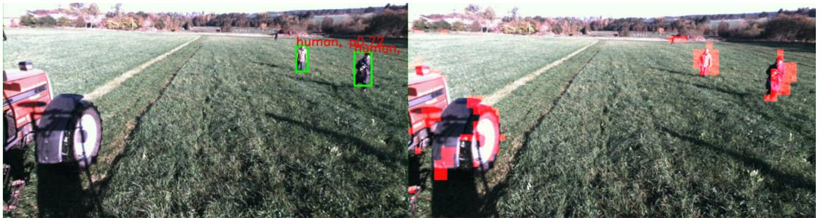
(4a) Object detection using YOLO.
