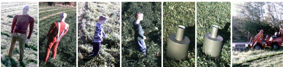
**Figure 6.** Examples of static obstacles.
