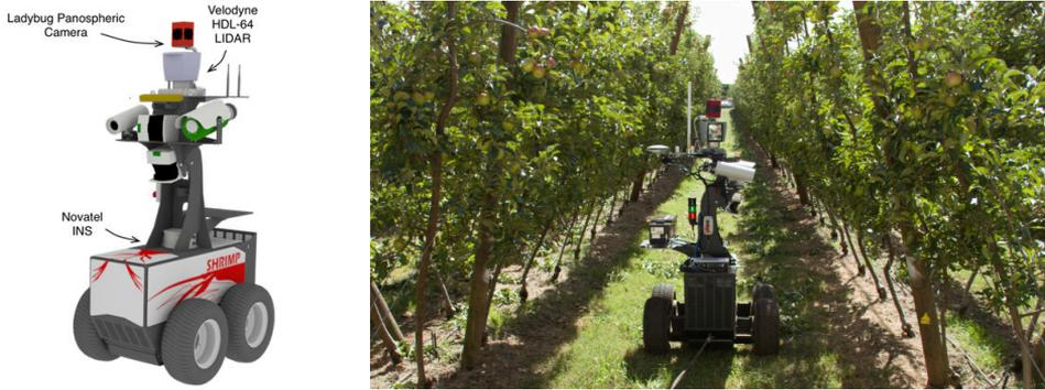
**Figure 7.** Robotic platform “Shrimp” with lidar, panspheric camera, and navigation system.
