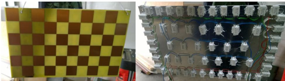
**Fig. 5** Front and back side of registration board
