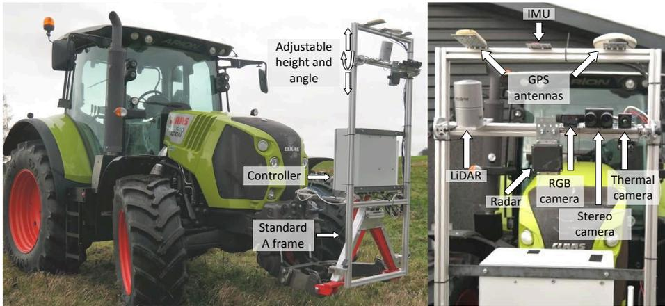
Figure 1. Sensor frame including controller.
