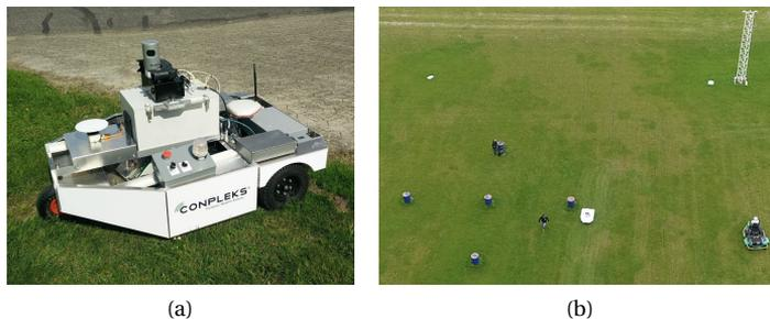
Figure 2.18: DK7: HCA Airport. (a) Sensors mounted on robot. (b) Drone image of robot and obstacles from above.
