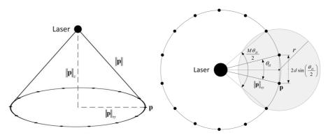
(a) Circular scan pattern on flat ground surface.
