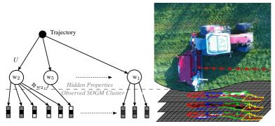
(7a) Conceptual representation of the proposed framework with the generative sampling on the left and a corresponding scenario with observations along the red tractor trajectory on the right.
