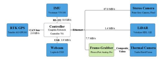
Fig. 2 System overview illustrating bandwidths and interfaces for sensors
