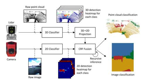
Figure 1. Schematic overview of fusion algorithm.
