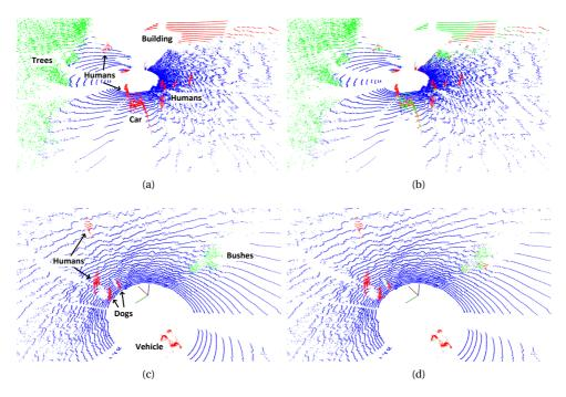
Figure 5.2: Examples of classification results. a) and b) respectively show ground truth and classification results of a scene with ground, trees, humans, a car, and a building. c) and d) respectively show ground truth and classification results of a scene with ground, bushes, humans, and dogs. Blue denotes ground, green denotes vegetation, and red denotes objects. Reprinted from Kragh et al. (2015).
