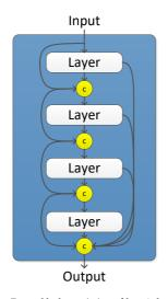
Figure 5: Dense block consisting of l = 4 densely connected composite layers.
