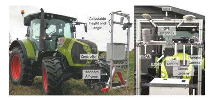
Fig. 1. Sensor platform mounted on tractor.
