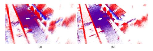
Figure 2.9: Georeferenced point clouds before and after optimization. (a) Handmeasured parameters. (b) Optimized parameters.
