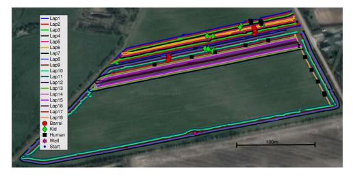
Fig. 4 Tractor route (*lines*), barrel (*circles*), kid mannequin (*diamonds*), adult mannequin (*squares*), well (*stars*) and lap starting point (*small dots*)
