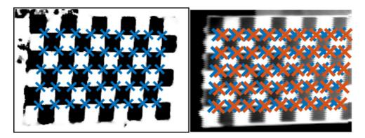
Fig. 14 Zoomed images. *Blue crosses* mark *corners* detected by the MATLAB calibration toolbox for both an RGB image (*left*) and a thermal image (*right*). The *red crosses* (*left*) show how 3D points are projected to the thermal camera (Color figure online)
