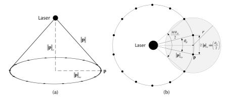
Figure 5.1: Example of adaptive neighborhood radius for single-beam lidar with M = 4. (a) Circular scan pattern on flat ground surface. (b) Overlaid adaptive neighborhood radius. Adapted from Kragh and Underwood (2017).
