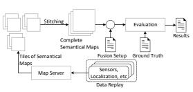
(9a) Evaluation pipeline from static recording to evaluation with stitching.
