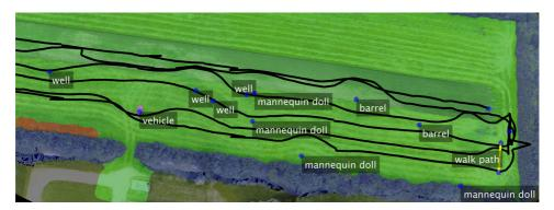
Figure 2.13: DK3: Foulum grass. Ground truth labels overlaid on orthophoto. The trajectory of the tractor is shown with a black line, whereas the walking path of a human is shown with a yellow line. The ground truth labels illustrate vegetation (blue), ground (green), and non-traversable ground (red). Adapted from Kragh et al. (2016b).
