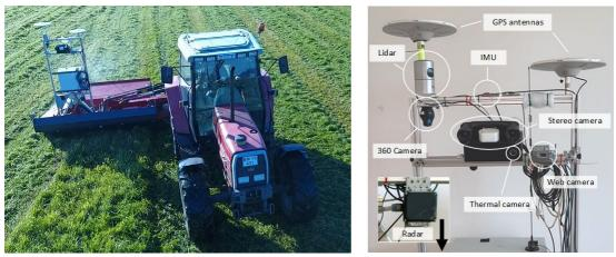
(2a) Platform attached to tractor-mounted mower.
