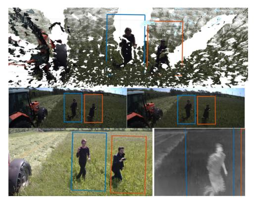
Fig. 8 Annotations in the *left image* are projected onto the stereo point cloud (*top*). These annotations are then projected to the right and left stereo camera (*middle left* and *right*), the webcam (*bottom left*) and the thermal camera (*bottom right*)
