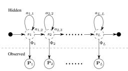
(7c) Left-right structure of one intra-property model  $\lambda_w$  for the inter-property model (exit transition per state is not visualized).
