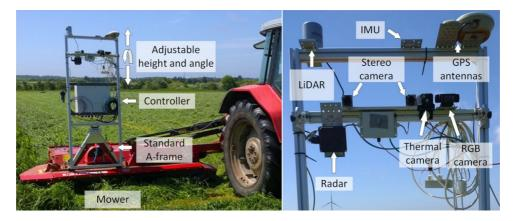
Fig. 1 Left sensor frame including controller. Right sensors on the sensor platform
