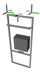
Figure 2.6: Simplified setup with only lidar, IMU, and GPS sensor frames.
