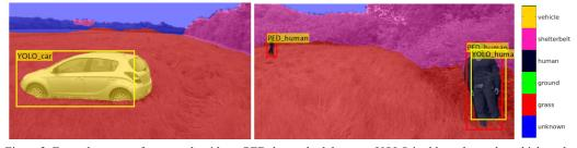
Figure 2. Example output of camera algorithms. PED detects both humans. YOLO is able to detect the vehicle and a human, but fails to detect the more distant human. SS detects both humans, the car, sky, ground and most of the shelterbelt. However, SS fails to detect the shelterbelt at far distance and around the human.
