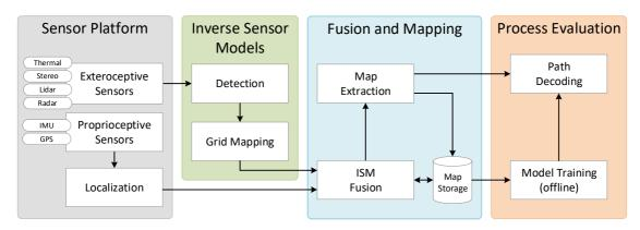
Figure 1. System architecture including information flow.
