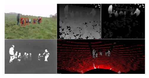
Figure 3. Detection of humans. RGB camera (top left), stereo camera disparity map (top middle), stereo camera protrusion map (top right), thermal camera (bottom left), LiDAR (bottom right).
