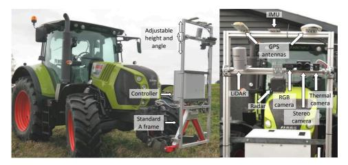
Figure 1. Sensor frame including controller.
