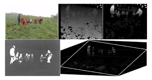
Fig. 9 Human detection. RGB (top left), stereo camera disparity map (top middle), stereo camera protrusion map (top right), thermal camera (bottom left), LiDAR (bottom right; Christiansen et al. 2015)
