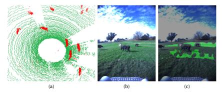
Figure 8.2: 3D ground segmentation and projection to 2D images. (a) ground and nonground 3D points. (c) 3D ground points projected on 2D image. (c) resulting pixel areas used for supervising the visual classifier.
