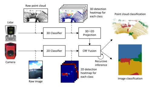
Figure 9.1: Schematic overview of proposed fusion algorithm. Reprinted from Kragh and Underwood (2017).
