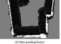
Figure 12.6: Example obstacle maps from static evaluation **A**. Intensities indicate occupancy probabilities with white being occupied, black unoccupied, and gray unknown. Red circles highlight static mannequin dolls in (a) and (b). Adapted from Korthals et al. (2018).
