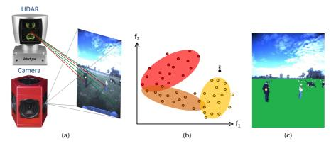
Figure 8.1: Camera-based traversability assessment supervised by lidar. (a) Lidar-classified ground and non-ground 3D points are projected onto 2D image.(b) Gaussian mixture model of normal ground appearance. (c) Ground truth traversable area overlaid on image.
