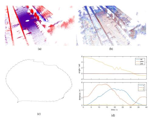
Figure 2.7: Georeferenced point clouds from subsequent lidar frames. (a) Accumulated points colored by height. (b) Voxelized point cloud colored by number of points inside each  $0.5 \,\mathrm{m} \times 0.5 \,\mathrm{m} \times 0.5 \,\mathrm{m}$  voxel. (c) Traversed circular path from above (d) Distance and angle coordinates as a function of time.
