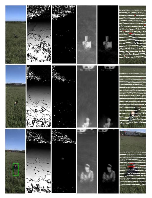
**Fig. 10** The three *rows* show respectively a barrel, a lying child mannequin and a sitting human. The *columns* show respectively pedestrian detections, a disparity map from stereo imaging, an object height map based on this, the thermal signature, thermal signature after subtracting the median temperature of the *bottom half* of the image, and the LiDAR projected onto the left stereo camera, where points protruding from the surface by more than 0.25 m are visualized
