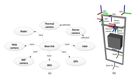
Figure 2.4: Sensor frames on the SuperSensorKit. (a) Registration chain. "Hand" denotes a manual measurement by hand, whereas "calibrated" indicates that an automated calibration procedure was used to estimate the extrinsic parameters.(b) Sensor frames overlaid on platform model. Adapted from Kragh et al. (2017).
