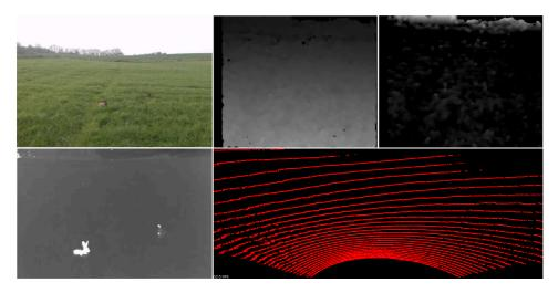
Figure 4. Detection of animals (rabbit and hen). RGB camera (top left), stereo camera disparity map (top middle), stereo camera protrusion map (top right), thermal camera (bottom left), LiDAR (bottom right).
