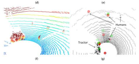
**Figure 3.** Example frames from the FieldSAFE dataset. (a) Left stereo image; (b) stereo pointcloud; (c) 360° camera image (cropped); (d) web camera image; (e) thermal camera image (cropped); (f) LiDAR point cloud (cropped and colored by height); (g) radar detections overlaid on LiDAR point cloud (black). Green and red circles denote detections from mid- and long-range modes, respectively.
