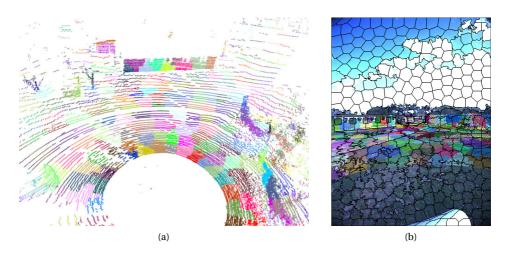
Figure 9.2: Segmentation in 2D and 3D. (a) Supervoxels in 3D. (b) Superpixels in 2D overlaid with projected 3D supervoxels. Adapted from Kragh and Underwood (2017).
