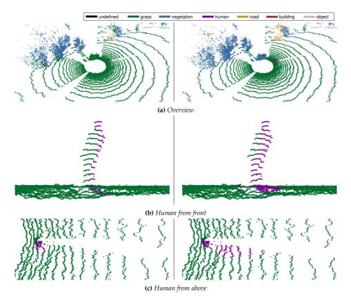
Figure 8: Three views on a single frame from the test set. The left column shows ground truth annotations, whereas the right column shows predictions using a network trained on range and intensity channels, only.
