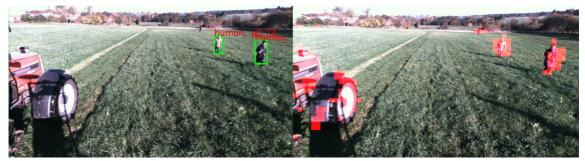
(4a) Object detection using YOLO.
