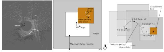
Figure 4. Left: Inverse sensor model as measurement grid of LIDAR for class "object". Center: Current patch as Region-Of-Interest. Right: Overlaid patches along a vehicle's trajectory
