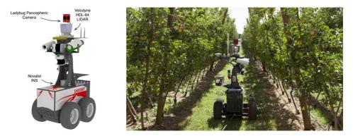
Figure 7. Robotic platform "Shrimp" with lidar, panospheric camera, and navigation system.
