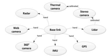
Figure 4. Sensor registration. "Hand" denotes a manual measurement by hand, whereas "calibrated" indicates that an automated calibration procedure was used to estimate the extrinsic parameters.
