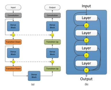
Figure 6.2: Network as proposed by Jégou et al. (2017). (a) Network architecture with concatenations denoted by o. (b) Dense block consisting of l = 4 densely connected composite layers. Adapted from Kragh et al. (2018).
