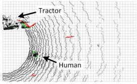
(6c) Radar detection example with confirmed (green) and unconfirmed (red) radar tracks overlaid on point cloud.
