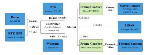
Figure 2. System overview illustrating bandwidths and interfaces between sensors, converters and the controller.
