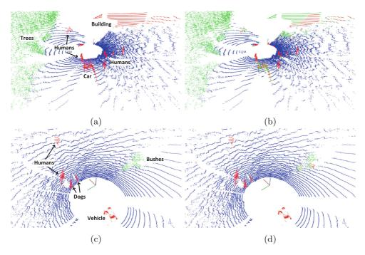
Fig. 2. Examples of classification results. a) and b) respectively show ground truth and classification results of a scene with ground, trees, humans, a car, and a building. c) and d) respectively show ground truth and classification results of a scene with ground, bushes, humans, and dogs. Blue denotes ground, green denotes vegetation, and red denotes objects (Colour figure online).
