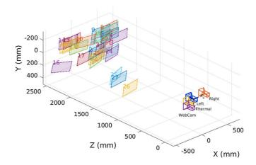
Fig. 7 Registration board placements (numbered 1-25) and inter-displacement of sensors
