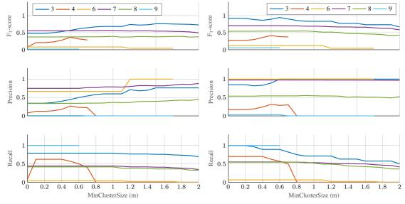
(10c) Precision, recall, and  $F_1$ -score over increasing minimum cluster size for different setups from Table 3. *ForgetRate* = 6 and *ForgetValue* = 0.8. Left: No dilation. Right: Dilation by vehicle radius of 2.5 m.
