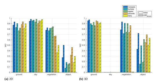
Figure 13. Classification results across object classes and datasets before and after sensor fusion.
