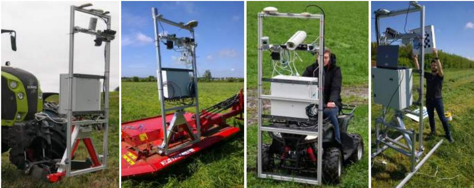
Figure 4.7: SuperSensorKit mounted on a tractor, implement, ATV and our lab mount.
