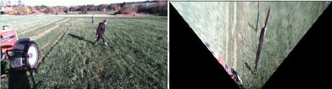
**Figure 6.** Inverse Perspective mapping of color image.
