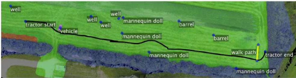
Figure 5.7: Orthophoto with static objects, tractor trajectory (black line) and human walk path (yellow line). An overlay shows the ground truth of shelterbelts (blue), ground (green) and non-traversable ground (red). From P[10]
