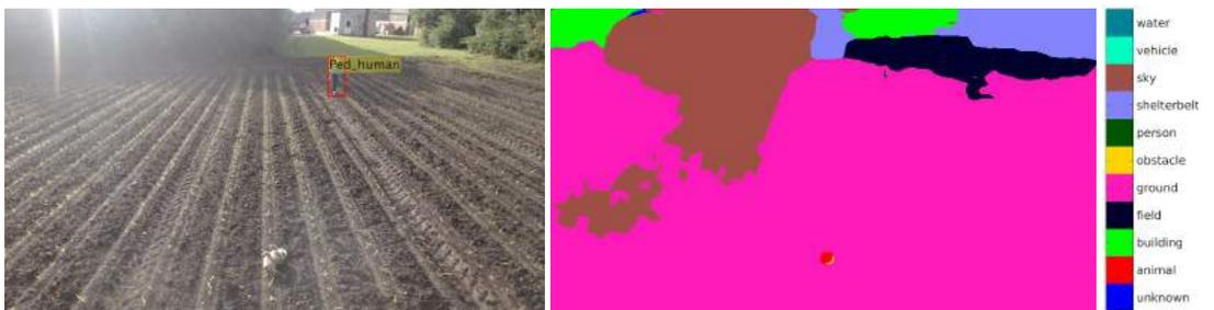
Figure 7. Test image in row crop. Semantic segmentation detects ground, shelterbelt, animal, field, building and just a bit of person. However, a large section of the field and shelterbelt is classified as sky and the dark area in the top left corner is classified as building. The top left corner - with very low contrast - is presumably classified as building as many
