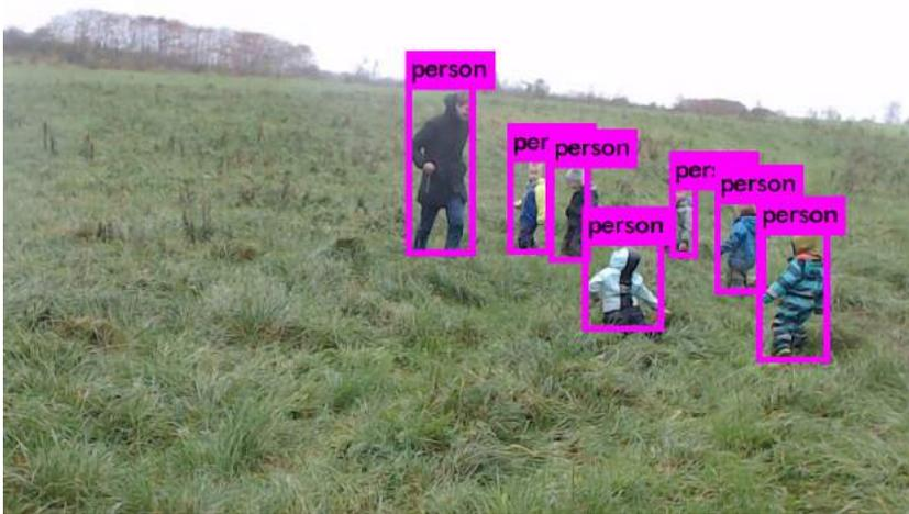
Figure 6.4: Hazard situation with YOLOv2. YOLOv2 is able to capable of detecting all persons including a falling kid.
