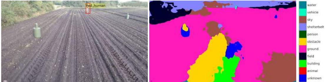
Figure 8. Test image in row crop. Large areas of shelterbelt and ground is classified correctly and the green barrels are classified as unknown or obstacles. The shelterbelt to the left is - as a reasonable guess - classified as field. However, large areas of ground are classified as obstacle, building and sky. The distant person is only detected by the pedestrian detector.
