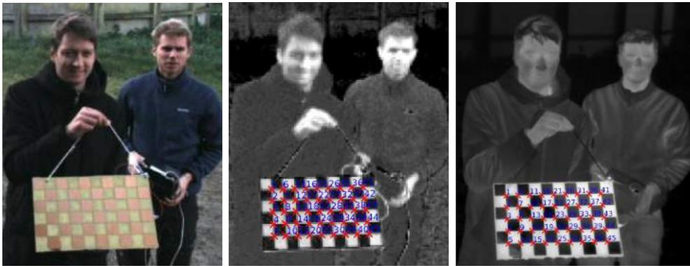
Figure 7.4: Thermal calibration panel as rgb, processed rgb and normalized thermal
