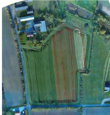
(a) Orthophoto with tractor tracks overlaid. Black tracks include only static obstacles, whereas red and white tracks also have moving obstacles. Currently, red tracks have no ground truth for moving obstacles annotated.
