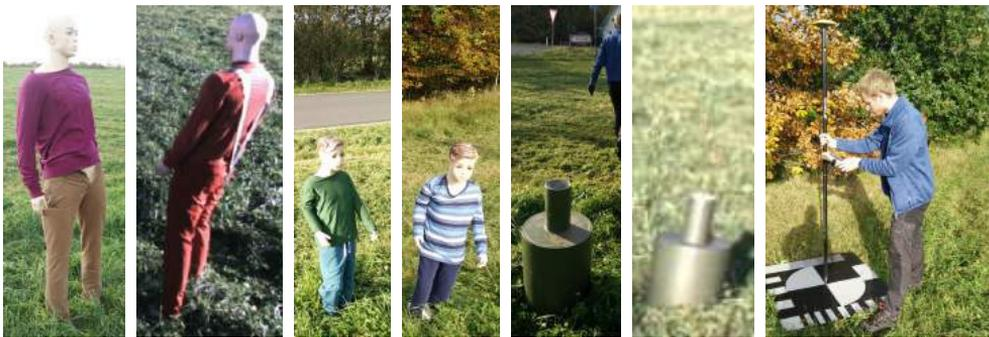
Figure 5.9: Static obstacles in the field. The position of GPS markers are measured using RTK GPS.
