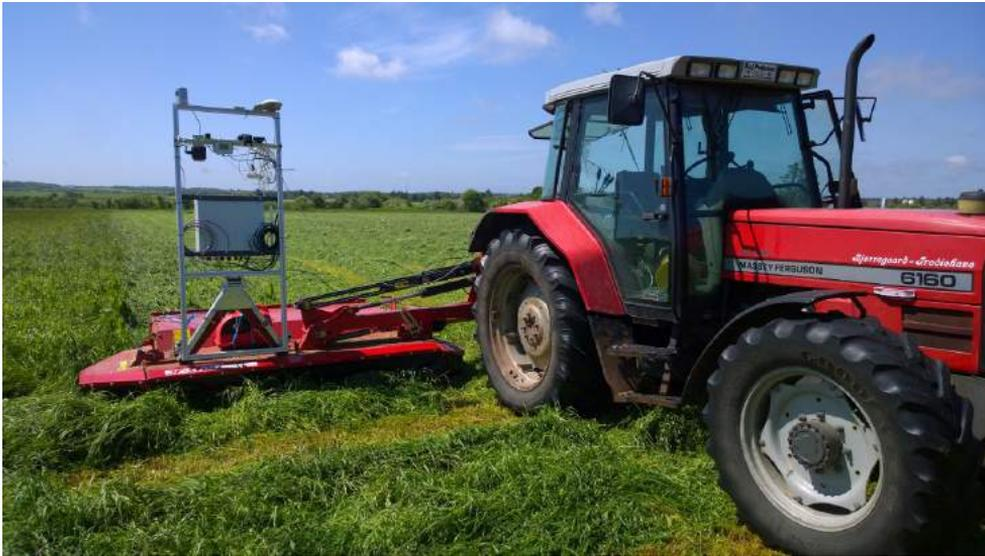
Figure 5.3: Tractor with implement and SuperSensorKit. From P[5]
