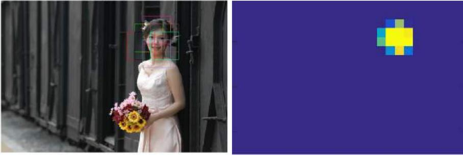
Figure 3. A fully convolutional neural network provides a grid of predictions or a heat map as output.
