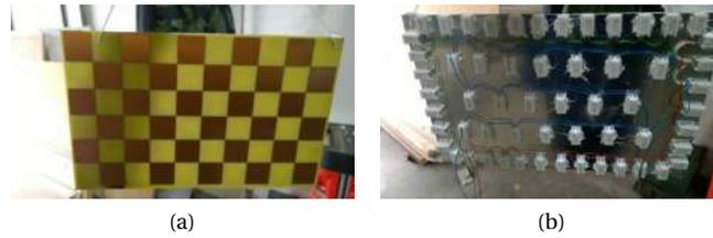
Figure 7.3: Front and back of thermal calibration panel. From P[6]
