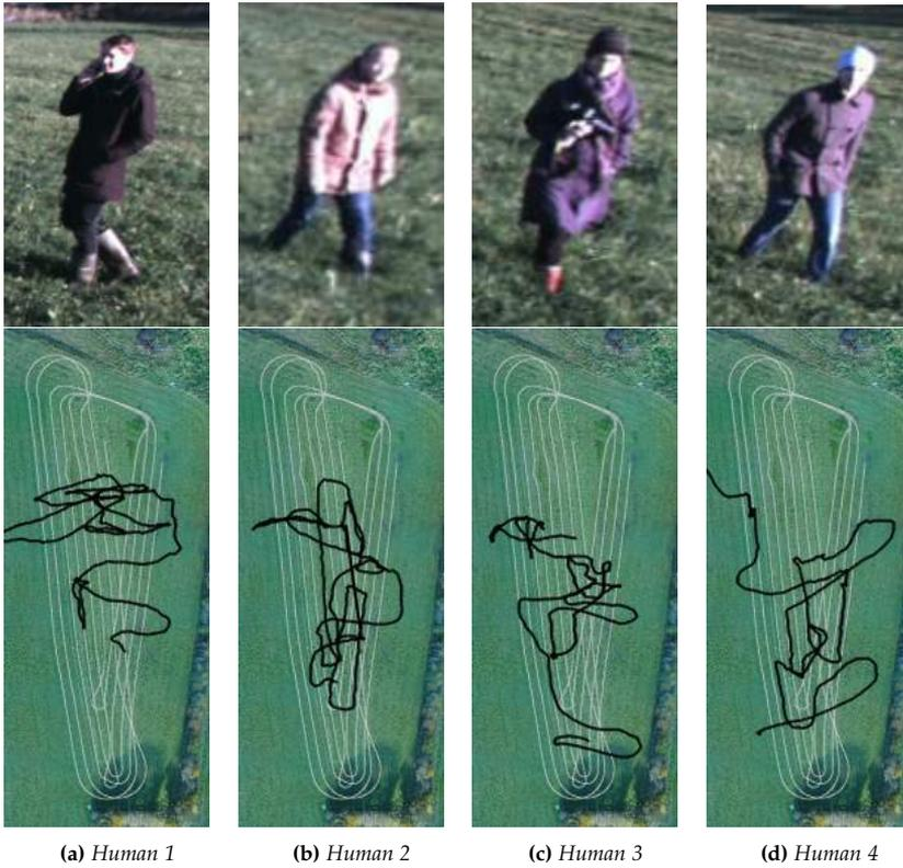
Figure 6: Examples of moving obstacles (from the stereo camera) and their paths (black) overlaid on tractor path (grey).
