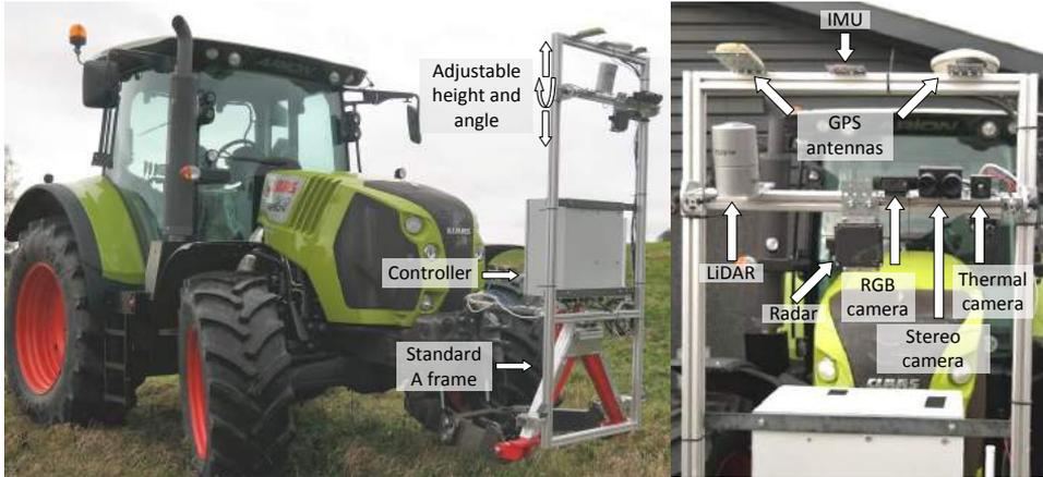
Figure 1. Sensor frame including controller.
