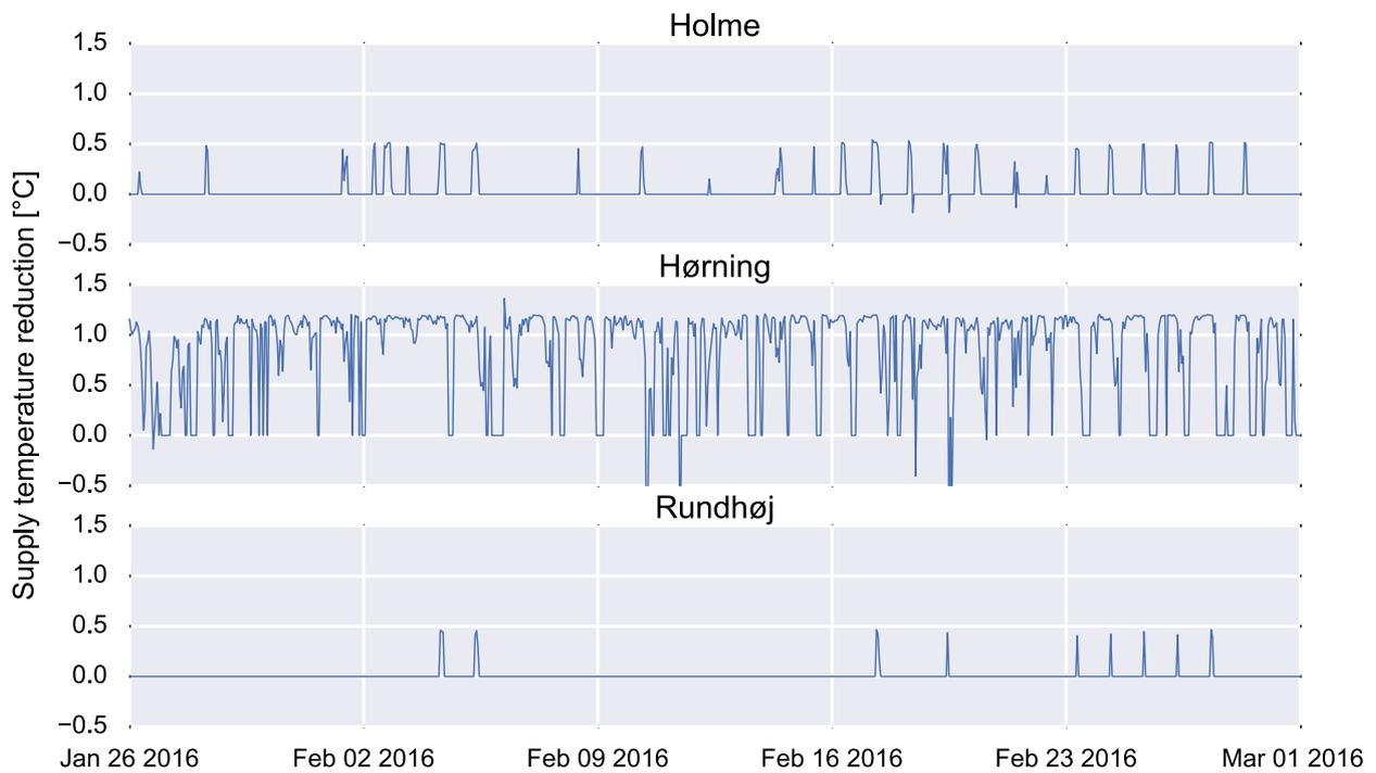
**Fig. 7.** Supply temperature reduction when switching from Scenario 2 to Scenario 3:  $T_{sup}^{Sc2} - T_{sup}^{Sc3}$ . This is shown for the three area substations Holme, Hørning and Rundhøj for the second half of the simulation period. For Hørning, the supply temperature in Scenario 3 is higher in a few time steps. This results in negative spikes in mid February reaching values down to  $-0.5$  °C to  $-1.6$  °C.
